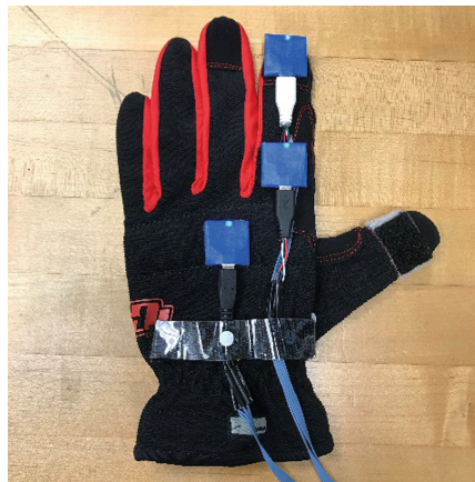
Fig. 2. The glove with IR-reflective dot markers attached on the wrist, one Yost Labs 3-space sensor attached on the back of the hand, and two Yost Labs 3-space sensors attached on the index finger
