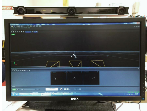
Fig. 1. The setup of OptiTrack V120: Trio with Motive:Tracker software
